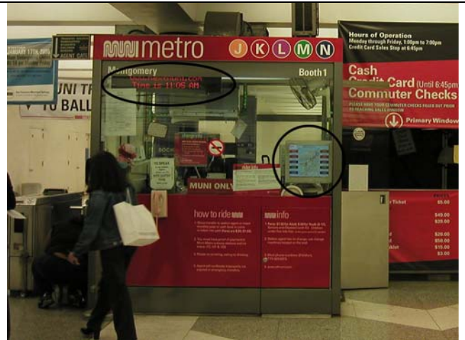
36. Muni agent booth. Note real-time information in lower right corner of window (circled). This technology was tested by Muni and is being replaced by NextBus technology. Display for this information, not yet active, is in upper left corner (oval).
