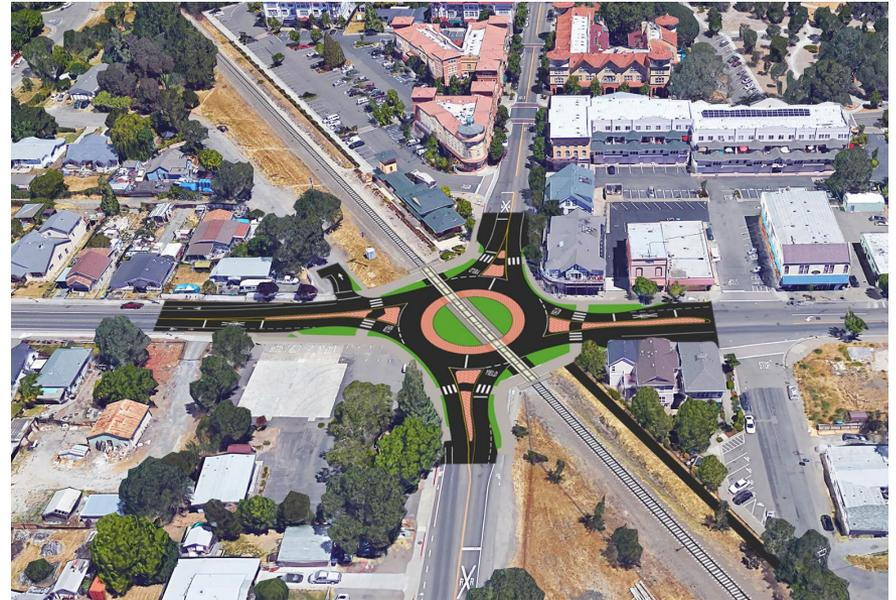
**Roundabout Option – would replace existing traffic signal and railway safety improvements would be added**
