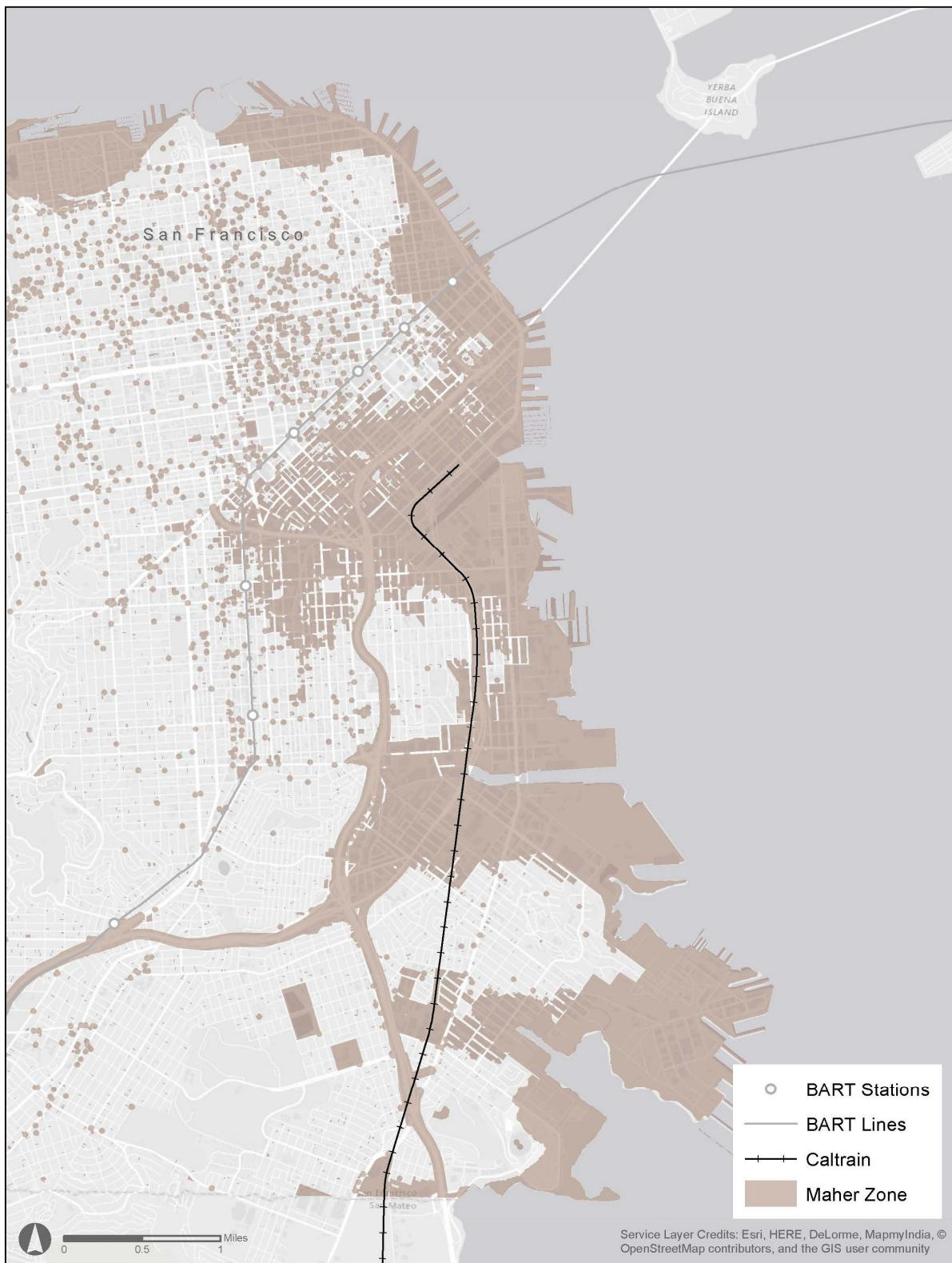
Figure A2. Maher zones in San Francisco – areas where fill soils contain potentially contaminated materials.
