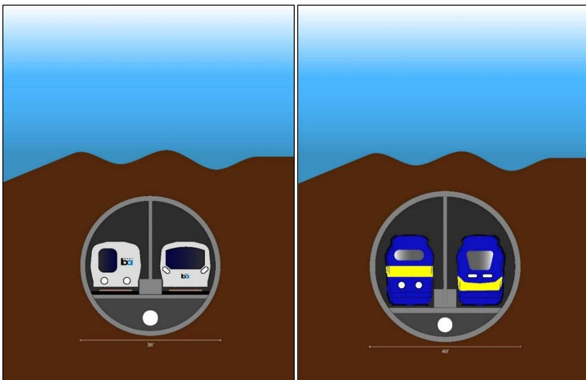
Figure A5. Schematic sections of BART and rail mined tunnel configurations.
