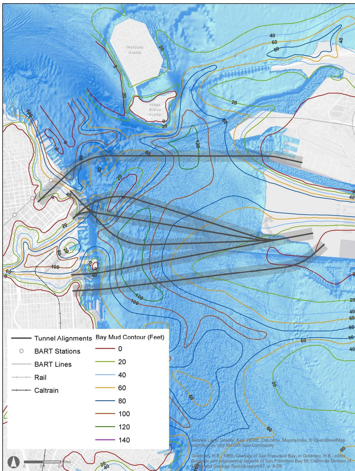
Figure A8. Potential tunnel or tube alignments in San Francisco Bay shown with bathymetry and approximate YBM thickness contours.
