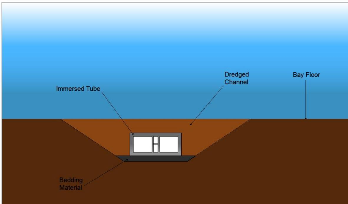
Figure A6. Two-track immersed tube construction schematic.
