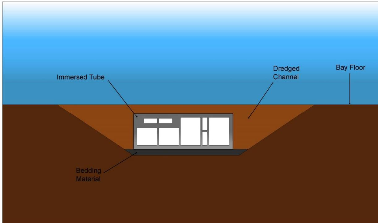
Figure A7. Four-track immersed tube construction schematic.
