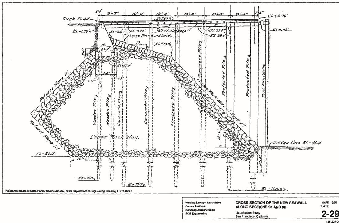
Figure A4. Cross Sections of the New Seawalls along Sections 9a and 9b showing Seawall piles extending to -71 feet (from HLA's 1992 Liquefaction Assessment Report).
