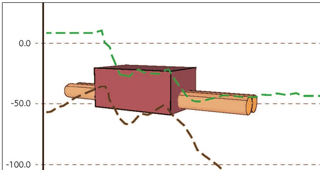
Figure A9. Surface stratigraphy (green), bottom of YBM (brown) shown with a schematic of an immersed tube (right) and transition structure. Where the structure is founded on YBM, ground improvement would likely be required. Cross section was cut approximately along the BART3 Alignment shown previous figures. Figure is not to scale.
