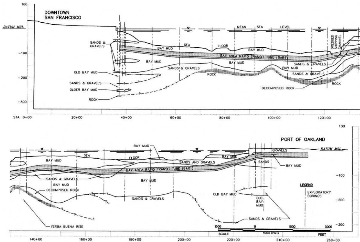
Figure A3. Interpreted Geotechnical Cross Sections of the Existing Transbay Tube Alignment across San Francisco Bay (from Parsons Brinkerhoff Quade and Douglas 1965).
