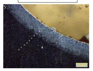
Vickers Microhardness measurement Locations, Specimen Center.
