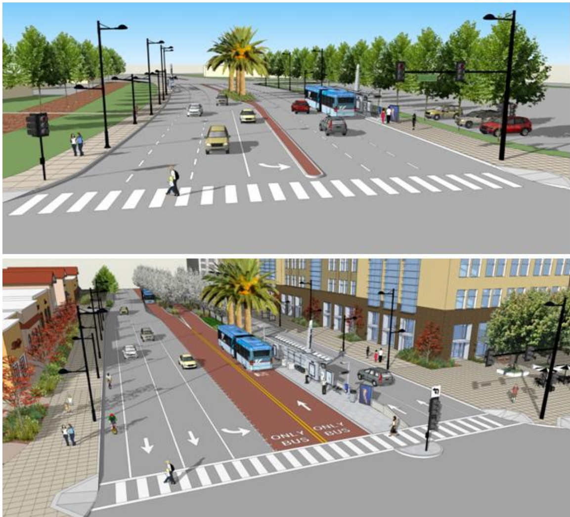
Figure 92 VTA BRT Concept Plans: Mixed Flow (top) and Dedicated Lanes (bottom)
