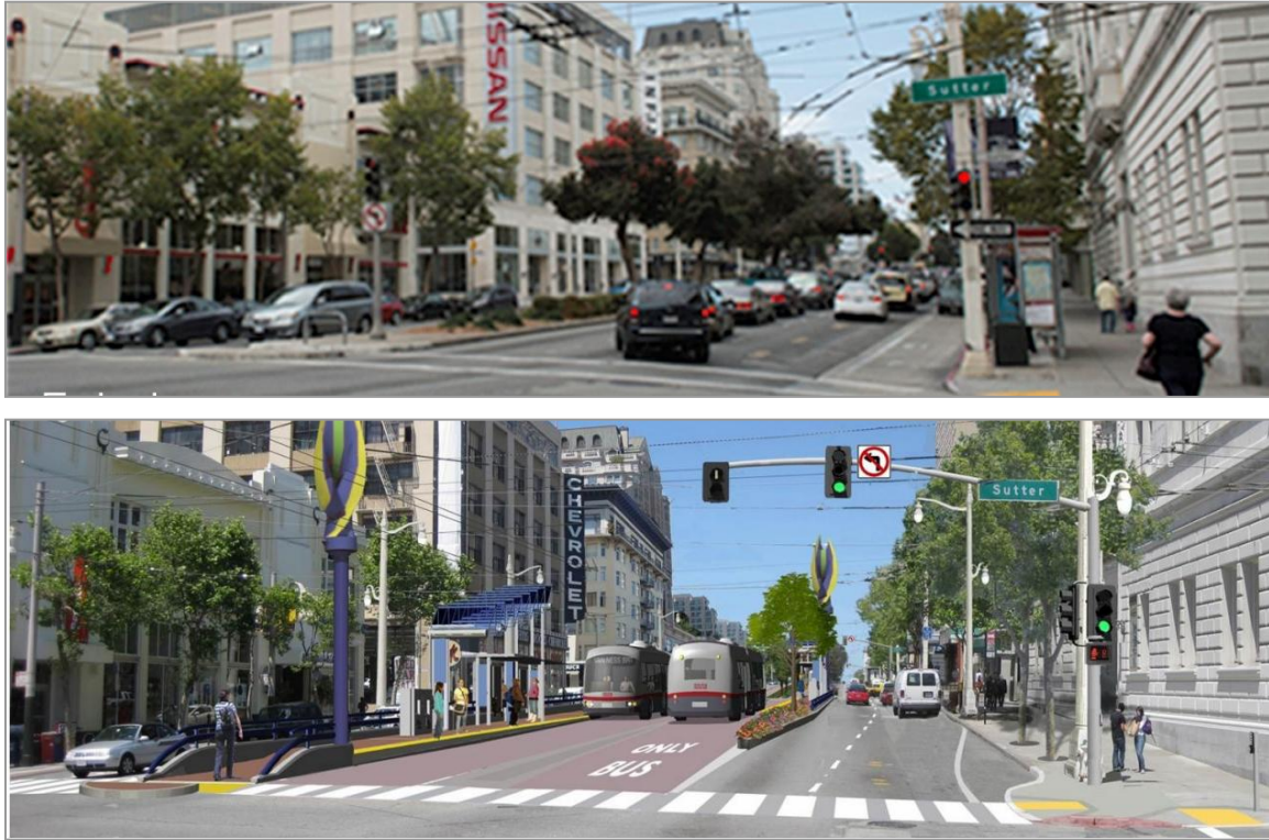
Figure 53 Van Ness BRT Design – Existing (Top) and Proposed (Bottom) Designs
