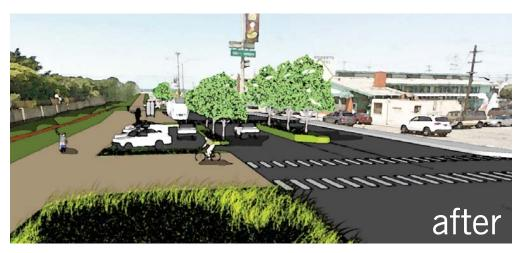
Figure V-4b: Proposed Sloat Blvd = Bike Lane + Pedestrian Walk + Diagonal Parking Pockets + 2 Driving Lanes + Planted Median + 2 Driving Lanes
