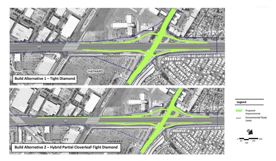
Figure 3. Build Alternatives at the I-880/Whipple Road-Industrial Parkway Southwest Interchange
